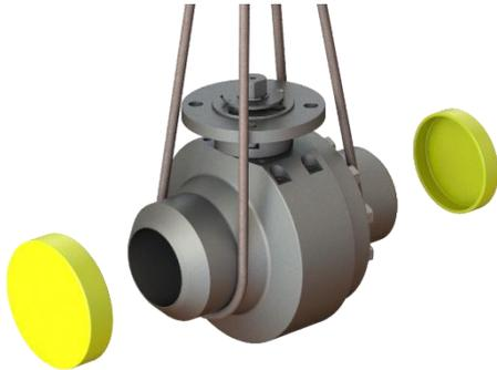
3. Clean the piping connection and the welding ends of the ARGUS Ball Valve.
