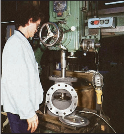
3 Relapping of seating faces after seal welding.
