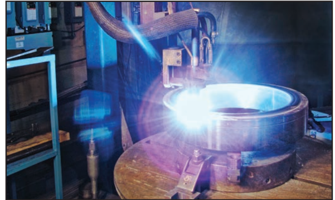
Automatic plasma arc hardfacing equipment for seats.
