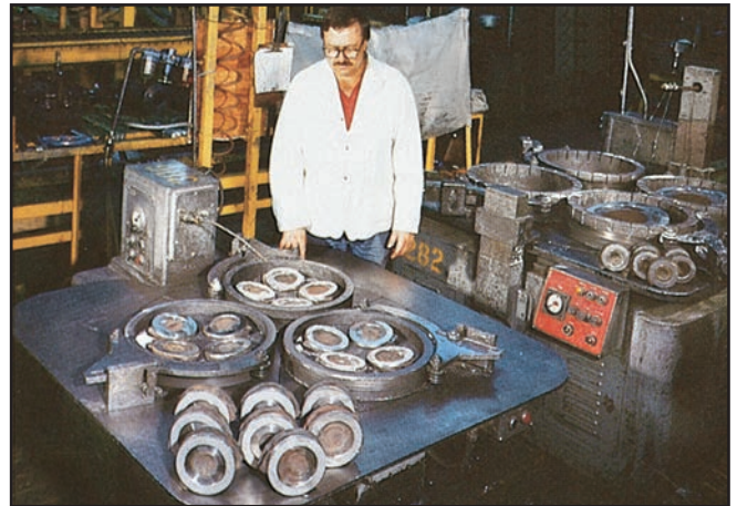
6 Lapping of wedge seating surfaces.
